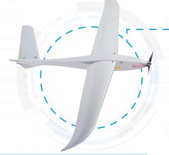
Take-off weight 5 kg Wing span 2600 mm 1250 mm Length Height 260 mm Flight duration 2h Communicational range up to 35 km Operational altitude 1000 m Stall speed 42 km/h Cruising speed 55 km/h Maximum flight speed 120km/h Sensor type FO camera Zoom 10x (optical)
