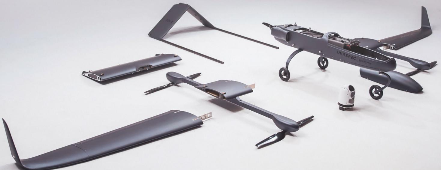
The PD-1 UAV can carry wide range of payloads, including EO/IR payload, radio intelligence unit, radio repeater, IMSI cell phone catcher or other equipment to support you operation. Huge payload compartment and 10 hours endurance with 10 kg payload give a lot opportunities for different applications.
