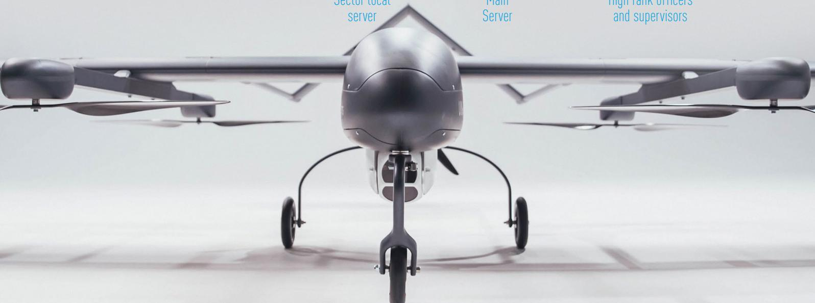
PD-1 platform easily handles ISR missions, artillery fire correction and general support missions. PD-1 UAV equipped with advanced EO/IR payload and stays in the air for up to 10 hours and has operating range of 400 km.
