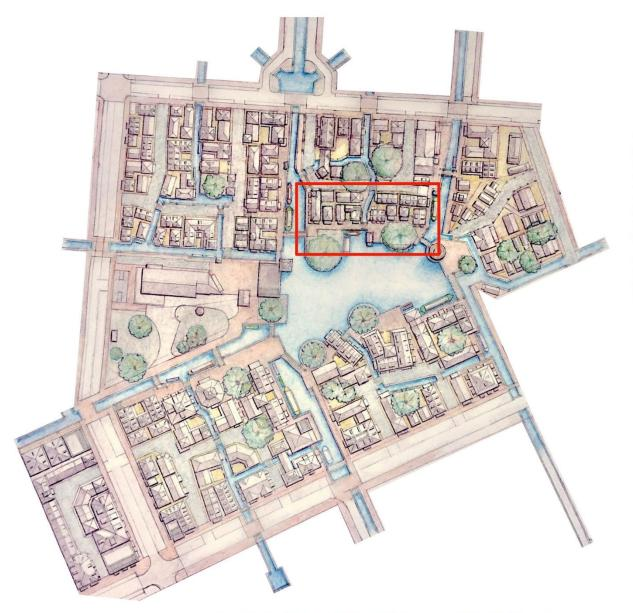
This preliminary draft of the Canal District Phase A.1 design uses the original I'on apartment units and Vince Graham's technique of unit plan cut-and-paste from the Mixon paste from the Mixon development. When maxing out the design it yields between 32 and 42 apartment/condo flats including 3 potential destination commercial shops. This is on just the 4 waterfront lots totaling 1/4 acre We are preparing a detailed pro forma.
