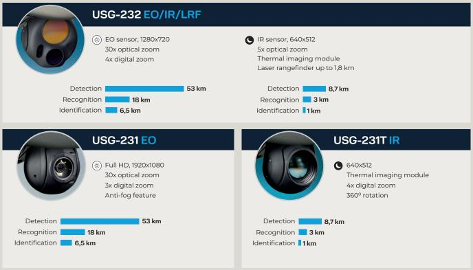
\*The DRI data for all cameras is specified for an object measuring 1.5 x 1.5 m under ideal weather conditions.
