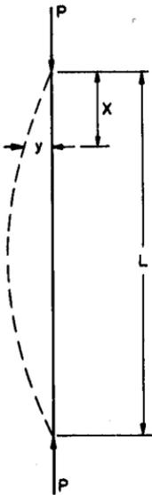
**FIGURE 5.43** Buckling of a pin-ended long column.
