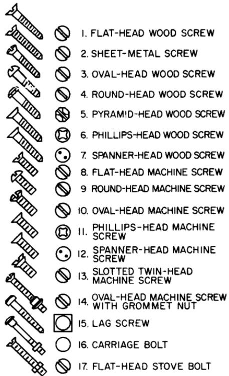
FIGURE 11.86 Typical screws.
