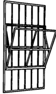
FIGURE 11.41 Security window with continuous muntins.
