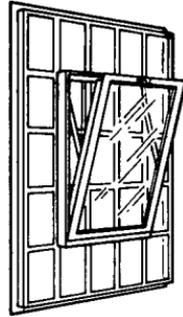
FIGURE 11.49 Guard-type detention window.
