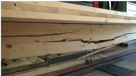
FIGURE 9: Typical bending failure in nonpretensioned T-sections corresponding to specimen F1/PIC-1.
