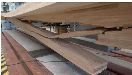
FIGURE 11: Failure close to a finger joint in the specimen F1/OAK-3.
