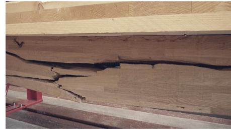
FIGURE 12: Bending failure in a pretensioned T-section corresponding to specimen F2/OAK-3.
