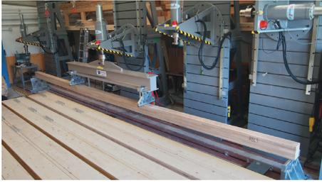
FIGURE 4: Bending test to determine the global bending MOE.
