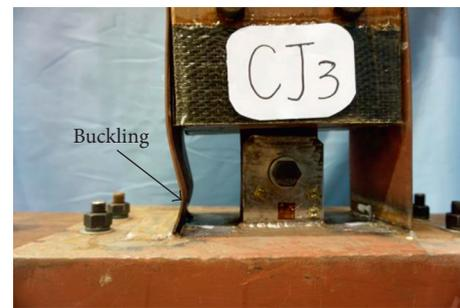
FIGURE 7: Beam flange buckled under compression for the specimen CJ3.
