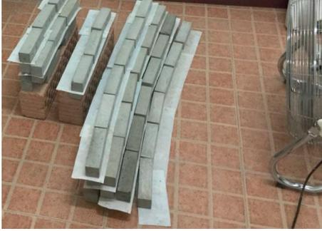
FIGURE 1: Water loss rate test of the DMPM prism specimen.
