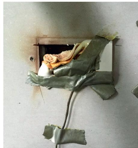
FIGURE 15: The external panel of the junction box softens at 28th minute in Test 2.
