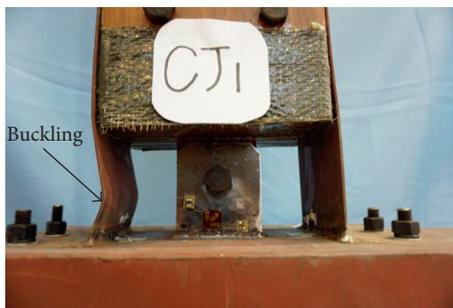
FIGURE 5: Beam flange buckled under compression for the specimen CJ1.
