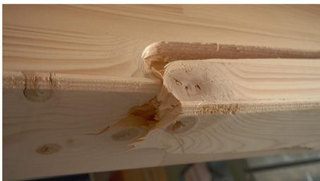
FIGURE 10: Failure due to knots in the specimen F1/PIC-3.
