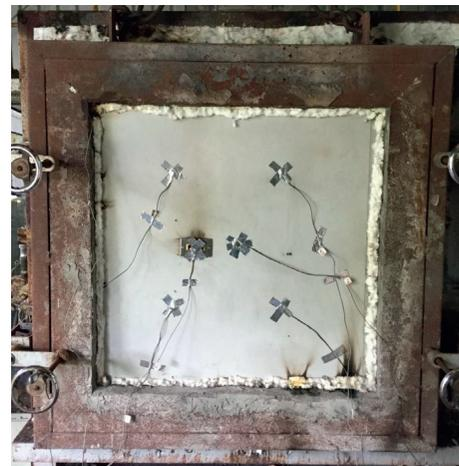
FIGURE 19: The result of the specimen after the 60 min standard fire test in Test 3.
