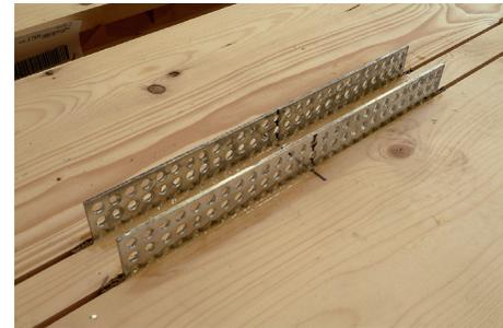
FIGURE 2: Discontinuous flange-to-web joint made with glued-perforated steel plates.
