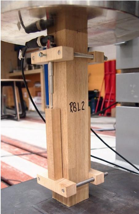
FIGURE 5: Test to determine the compression MOE parallel to the grain.
