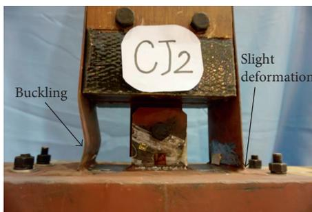
FIGURE 6: Beam flange buckled under compression for the specimen CJ2.
