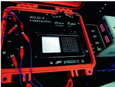
FIGURE 3: Soil resistivity acquisition instrument.
