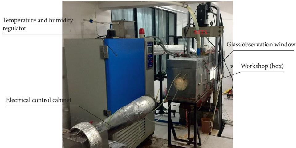
FIGURE 2: Intelligent environment simulation and controlling system.
