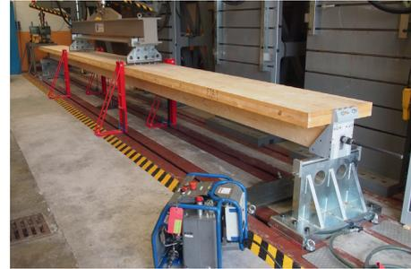
FIGURE 6: Test of a pretensioned T-section with *Picea abies* webs.
