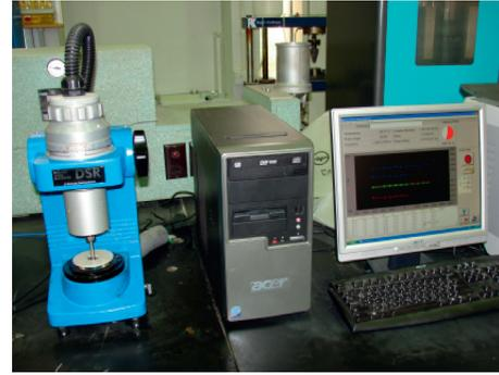
FIGURE 2: Dynamic shear rheometer (DSR).
