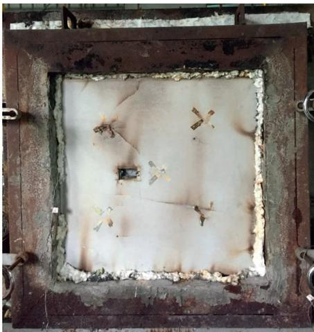
FIGURE 17: The result of the specimen after the 60 min standard fire test in Test 2.
