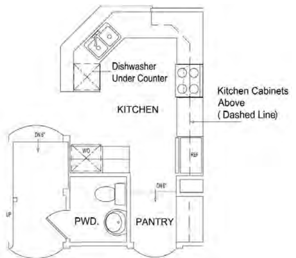
Figure 3.3B Hidden lines here represent an undercounter appliance and hung kitchen wall cabinets.
