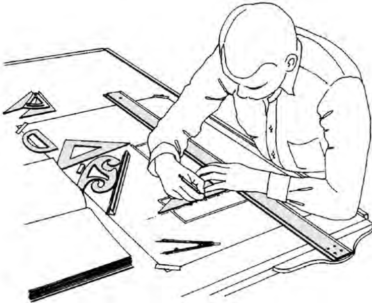
Figure 2.1 A drafter using a typical drawing board, t-square, and other instruments (after Muller, Edward J., et al.: Architectural Drawing and Light Construction , 5th ed., Englewood Cliffs: Prentice Hall, 1999).
