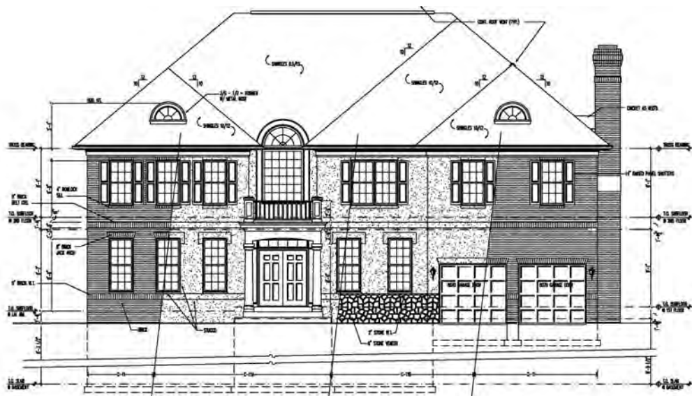
FRONT ELEVATION C-11 SCALE: 1/4" = 1'-0"
