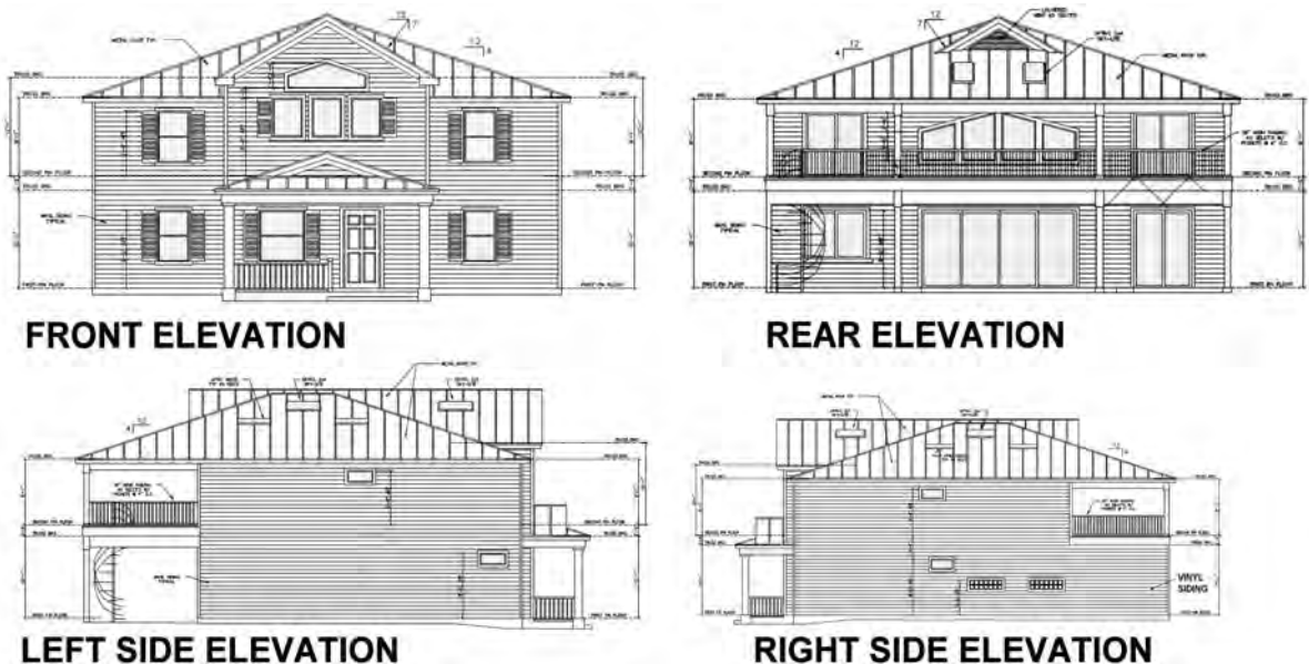
Figure 6.12A Four exterior elevations of a house will normally accurately depict its features, including materials used and vertical heights.
