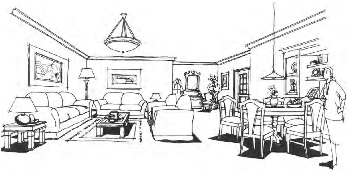
Figure 5.25A A. Illustration of an interior using normal-view one-point perspective.
