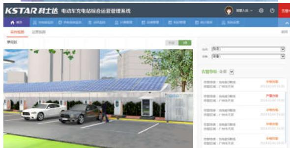
Appearance of charging station displayed by 3D view, as if observing charging station on the scene so as to find out the area with alarm in time
