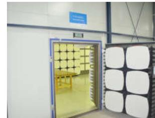
EMI laboratory (for measurement of RE radiated interference)
