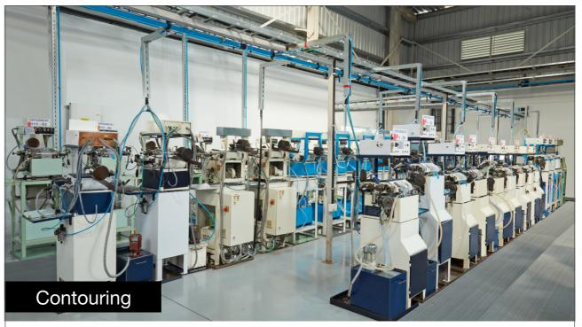
There are 45 contouring machines which have got the capability to contour variety of configurations such as circular, squares, rectangular, oval, and all odd shapes. Machines can give any configuration
