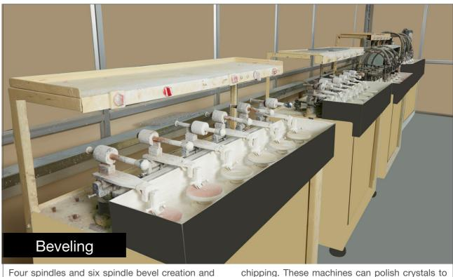
Four spindles and six spindle bevel creation and polishing machines that create a single or double side, 45 degree polished bevel that is free of edge within 20 microns accuracy and shape crystals of 4 mm to 70 mm in diameter. These machines also create negative radius. They can handle glass of thickness ranging from 0.8 mm to 5.00 mm.
