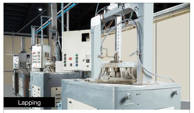
Five double side lapping machines are used to bring crystals to desired thickness and the parallelism. The accuracy achievable in thickness is 10 microns and the parallelism better than 3 arc minutes. Working range is from 4 mm to 70 mm in diameter.
