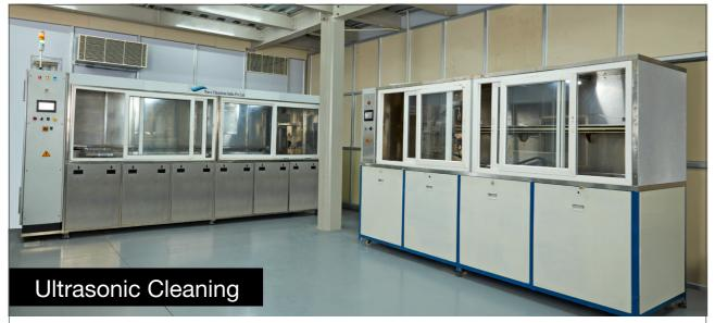
To manufacture the highest quality crystals four automated ultrasonic cleaning machines are established to ensure crystals are free from oil, cerium oxide and other contaminants. These machines are used at several stages of crystal manufacturing.
