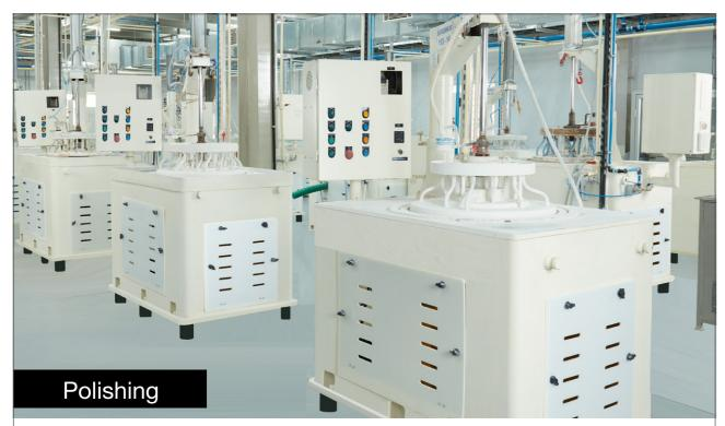
Sixteen double side surface polishing machines with variable speed and pneumatic pressure are used to work on flat crystals. These machines can create polished surfaces without any scratches and sleeks meeting Horological standards. To work on curved crystals several cylindrical polishing machines are available.
