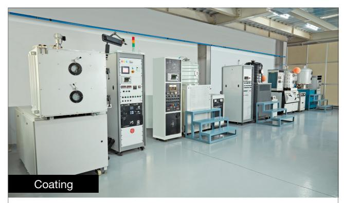
Four customs designed coating units metallize custom colours and standard colours such as gold, silver, rose gold and dark grey. The entire coating process is automated. Our coatings
