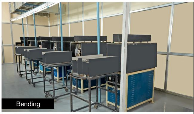
Six optical and vacuum bending machines bend plain glasses to different radius of domes.
