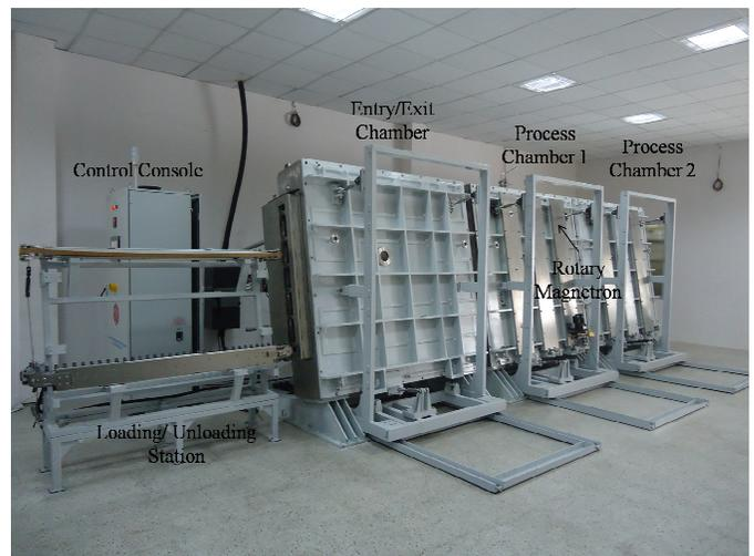
**Figure 1.** Rotary Magnetron Sputtering system developed by HHV for large area AZO coatings.
