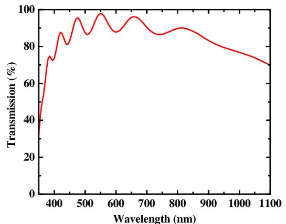
**Figure 3.** Transmission spectrum (glass compensated) for the optimized AZO coating.
