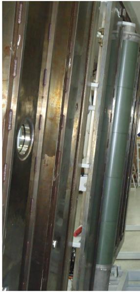
**Figure 2.** The inside view of the system showing the rotary magnetron mounted on to the chamber door.
