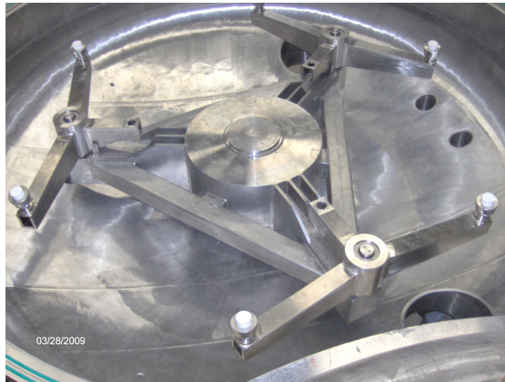
Figure 3. Rotatable Whiffle tree.
