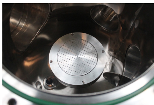
Showerhead electrode for PECVD
