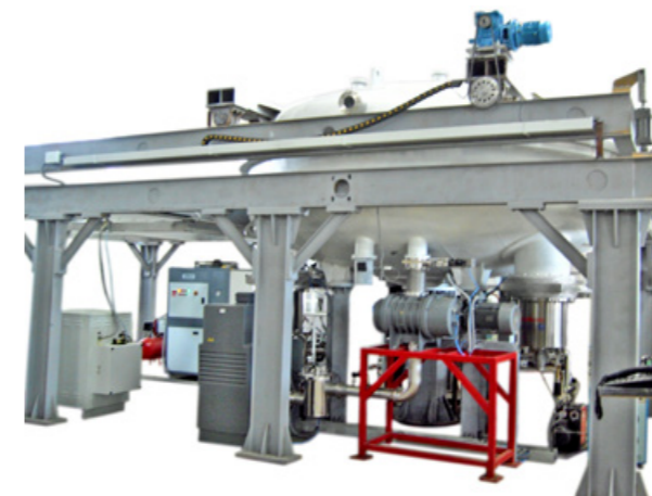
ARIES HHV sputter coater for 3.7 m diameter telescope mirror and chamber interior showing whiffle tree mirror support.
