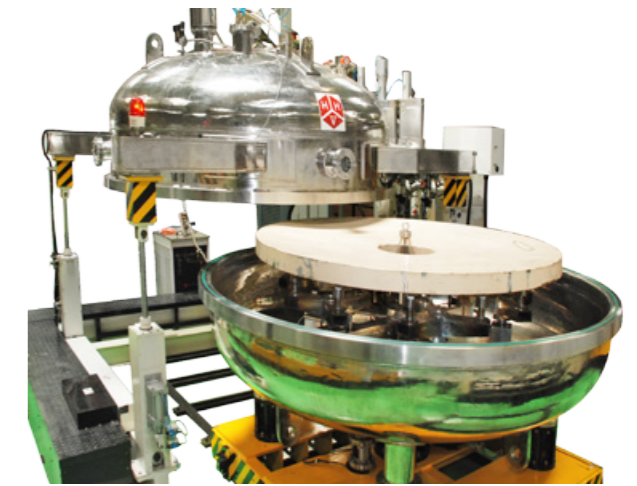
IIAP 2.1 m diameter mirror coater with PC SCADA control; Lower chamber in the load/unload position; and coater system fitted with mirror test blank.
