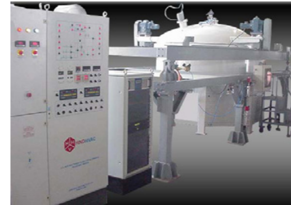
IUCAA Sputter Coater for 2.2 m diameter Telescope Mirror.
