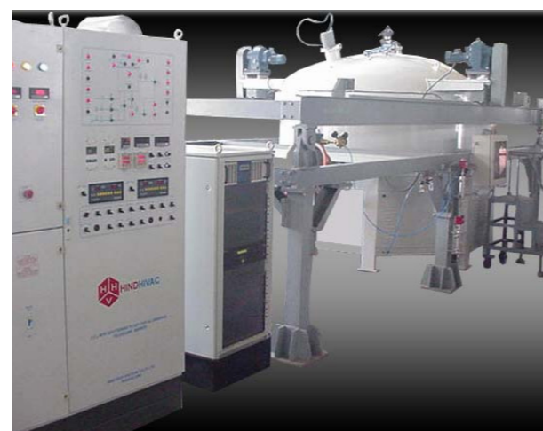
Sputter Coater for 2.2 m diameter Telescope Mirror for IUCAA.
