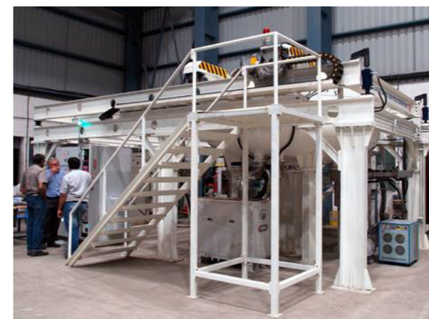
HHV astronomical telescope mirror sputter coating system installed at Caucasus Mountain observatory, Sternberg Astronomical Institute, Russia.
