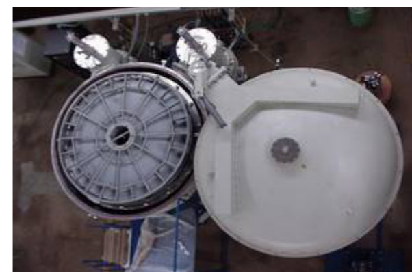
Evaporation coater for 2.1m diameter Telescope Mirror for IIAP.
