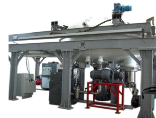
Sputter coater for 3.7 m diameter telescope mirror for ARIES.
