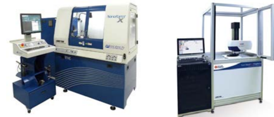
Figure 2: Nanoform machines for machining and Taylor Hobson for metrology
