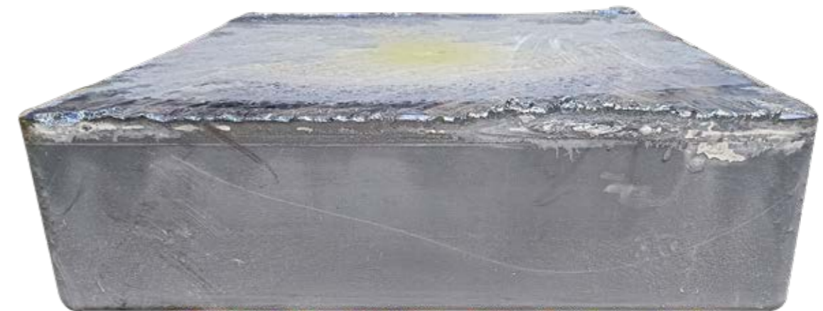
Figure 2: Multi-crystalline ingot of 800 Kg
