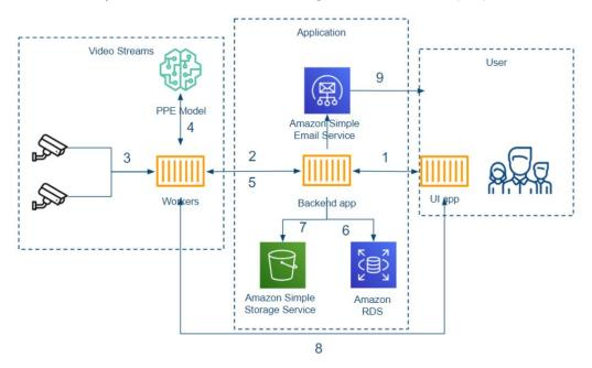
The architecture consists of three parts: User UI, Application backend, and Video streams processing using machine learning. Here's how it works:
