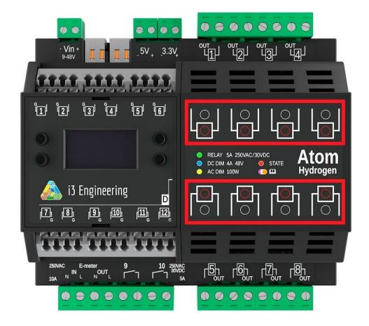
Output status indicator - red LED that displays the active output status of the controller;
