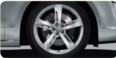
Audi Sport cast aluminium wheels in 5-spoke blade design size 9 J x 20 with 265/40 R 20 tyres 1 . From quattro GmbH
