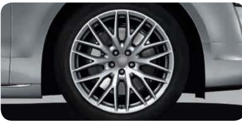
Audi Sport cast aluminium wheels in 10-Y-spoke design size 9 J x 20 with 265/40 R 20 tyres 1 . From quattro GmbH
