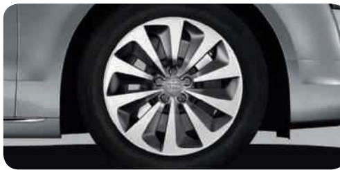
Cast aluminium wheels in 10-arm turbine design (hybrid design), contrasting grey, partly polished 2 size 9 J x 19 with 255/45 R 19 tyres 1 . Available only for the A8 hybrid and A8 L hybrid
