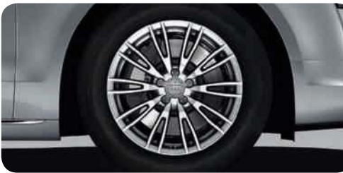
Cast aluminium wheels in 10-spoke V design size 8 J x 18 with 235/55 R 18 tyres 1
