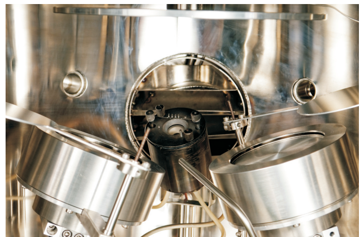
ATS 500 chamber with two 100mm sputter sources & ion beam source
