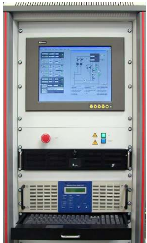
TF600 rack with PC control for fully automated system and process operation
