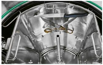
A creative and adaptable evidence holder made of magnetic stainless steel that is semicylinder in shape To make attaching the evidence to the holder easier, it can be turned to different angles and retracted from the chamber.
