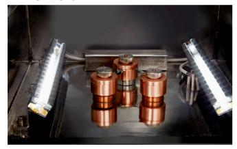
Internal LED lighting is installed in the vacuum chamber so that the operator can watch and keep an eye on the process. The touch screen controls the lighting
