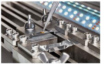
The evaporation sources are positioned on circular copper busbars that are centered. The system is quite versatile because of its creative design, which allows the user to deposit a combination of three metals—gold, zinc, and silver—in a single deposition process. Depending on the size of the evidence, the source placements can be adjusted to maximize the coating performance.
