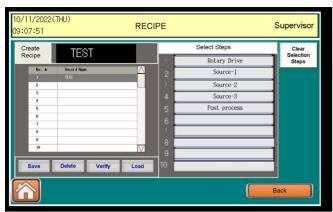
Recipe based coating cycles includes automatic control of the pumping system, deposition source, Rotation
