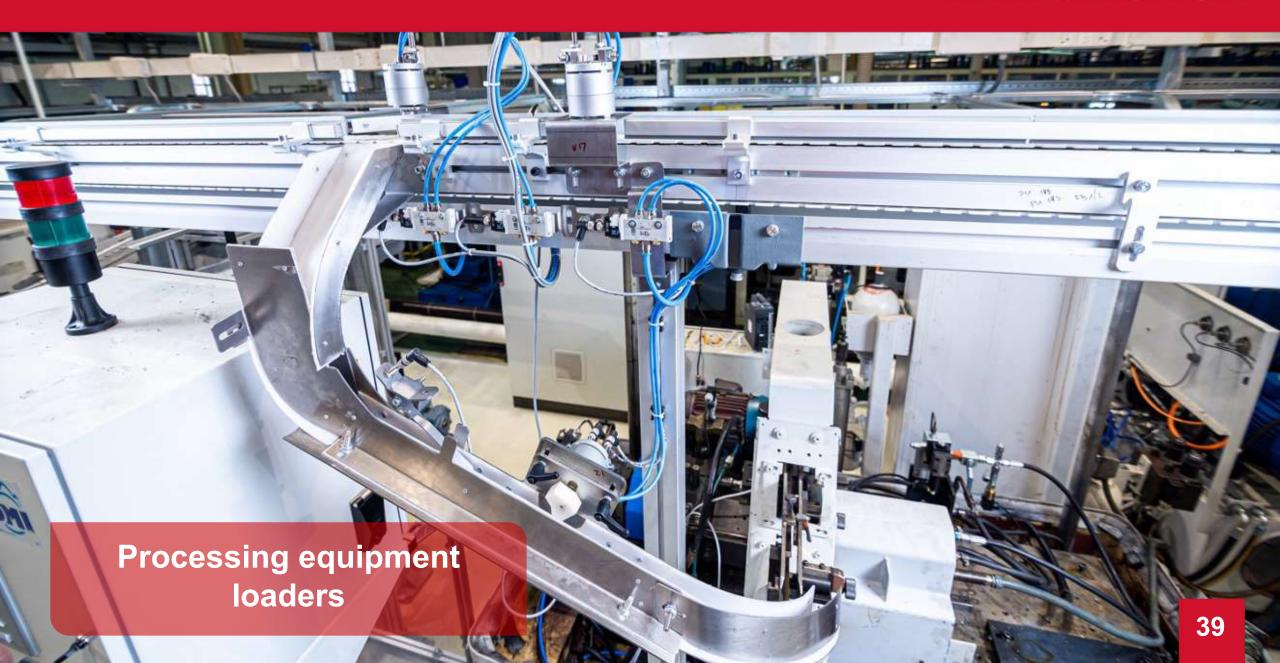
Ring position check and and loading mechanism
