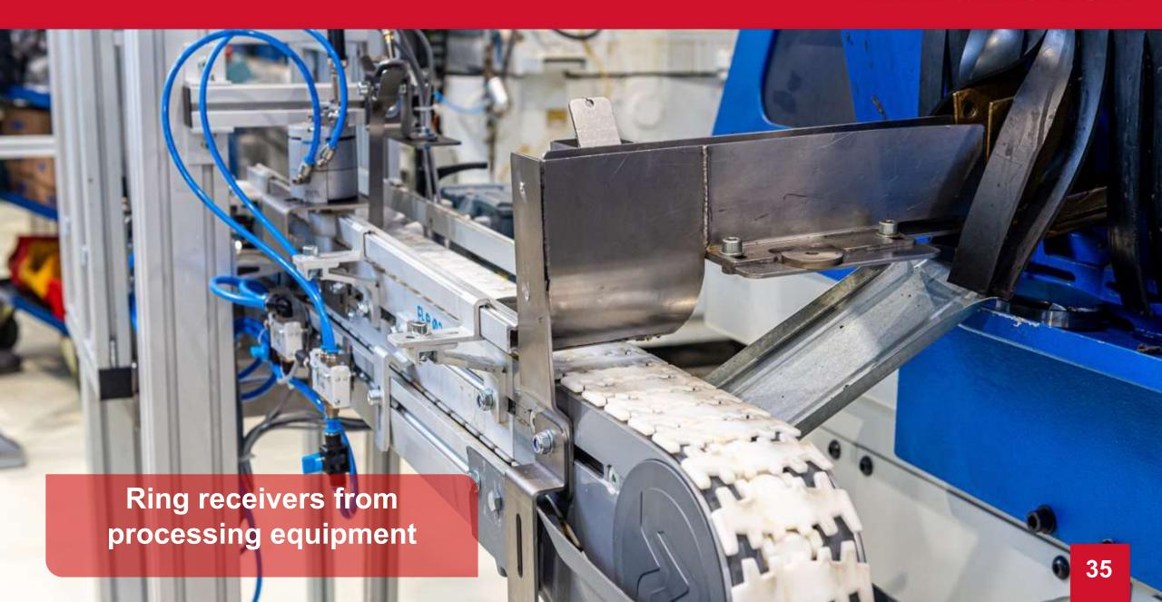
Ring position check and rotation module in action
