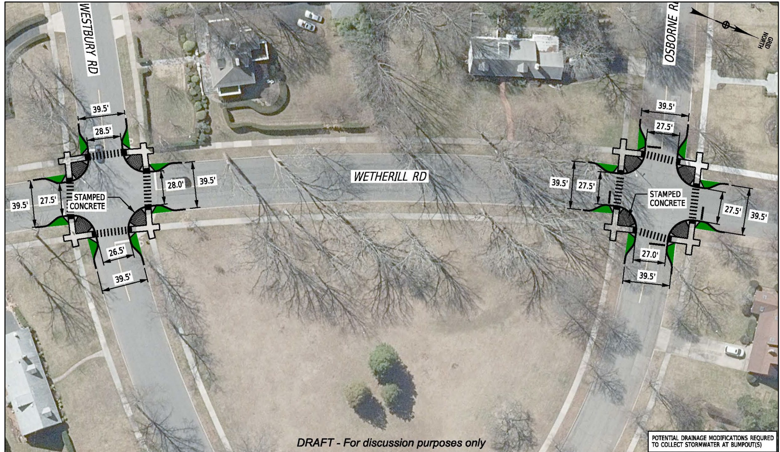
Sketch plan showing intersection bump-puts on Wetherill Rd at Westbury Rd and Osborne Rd near Triangle Park
