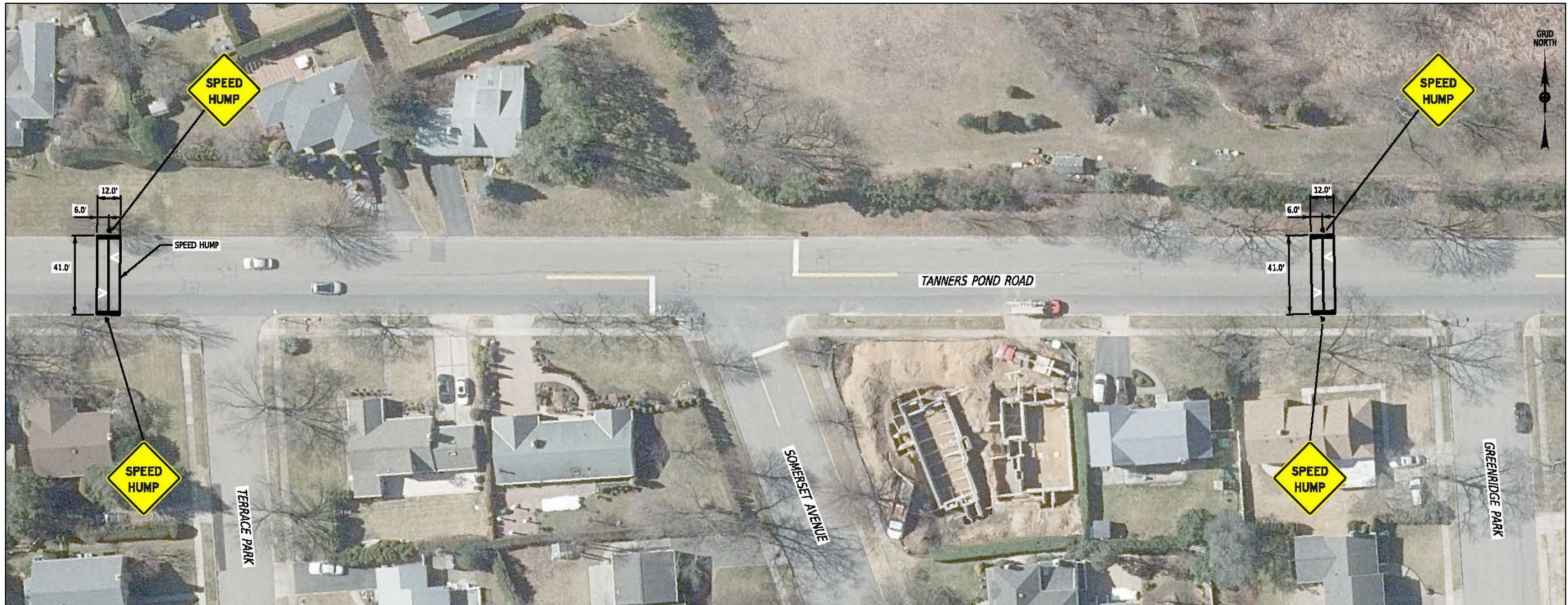
Figure 38: Sketch plan showing multiple speed humps along Tanners Pond Rd with schematic to show vertical profile
