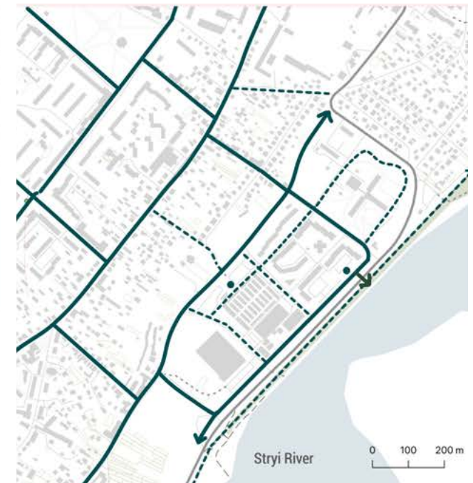
Figure. 46 Layout of cycling infrastructure Source: Ro3kvit
