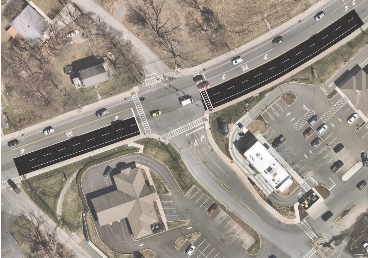
FIGURE 3.4: HOOSICK ROAD WIDENING AT ROOSEVELT AVENUE
