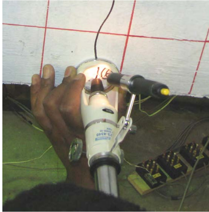
Figure S.2 Hand optical microscope for measuring initial crack-width (See Clause S.4.8 and S.7.2. )
