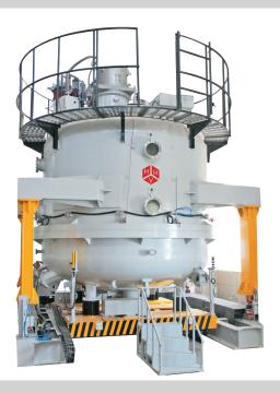
Telescopic mirror coaters for deposition of Aluminium and protected Silver coatings for astronomical applications
