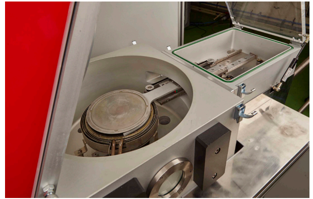
Telescopic arm for transfer of substrates between load-lock and process chambers.
