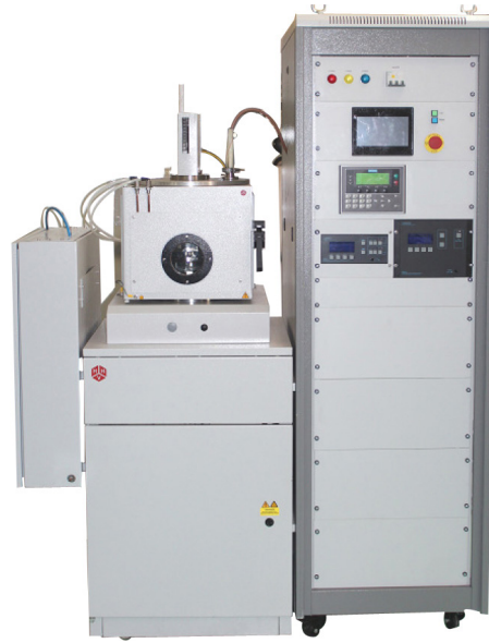
System configuration with integrated gas manifold
