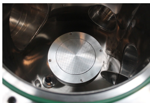
Showerhead electrode for PECVD
