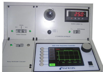
Quartz crystal monitor based control
