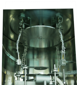
Rotary work holder with heater
