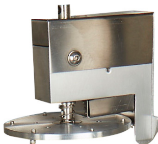
Glancing angle deposition (GLAD) work holder
