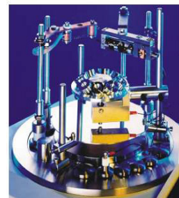
Rotatilt work holder
