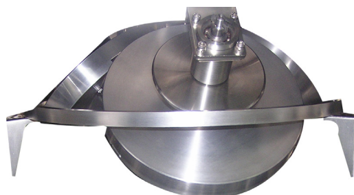
Knudsen planetary work holder
