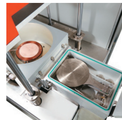
Reactor with load lock chamber
