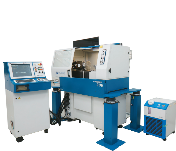
Figure 1: Nanoform systems for Single Point Diamond Turning
