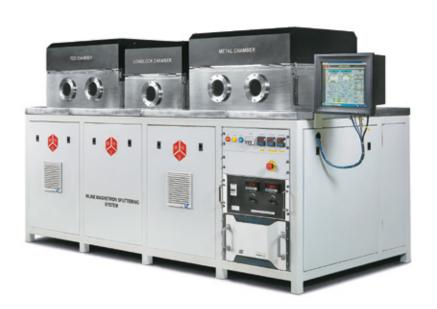
In-line magnetron sputtering system is a model platform for upscaling technologies and pilot scale production
