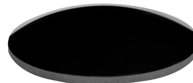
Fig.2. Chalcogenide components coated with ARC
