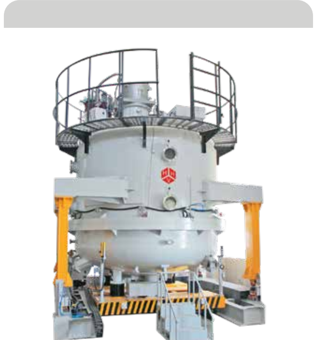
Telescopic mirror coaters for deposition of Aluminium and protected Silver coatings for astronomical applications
