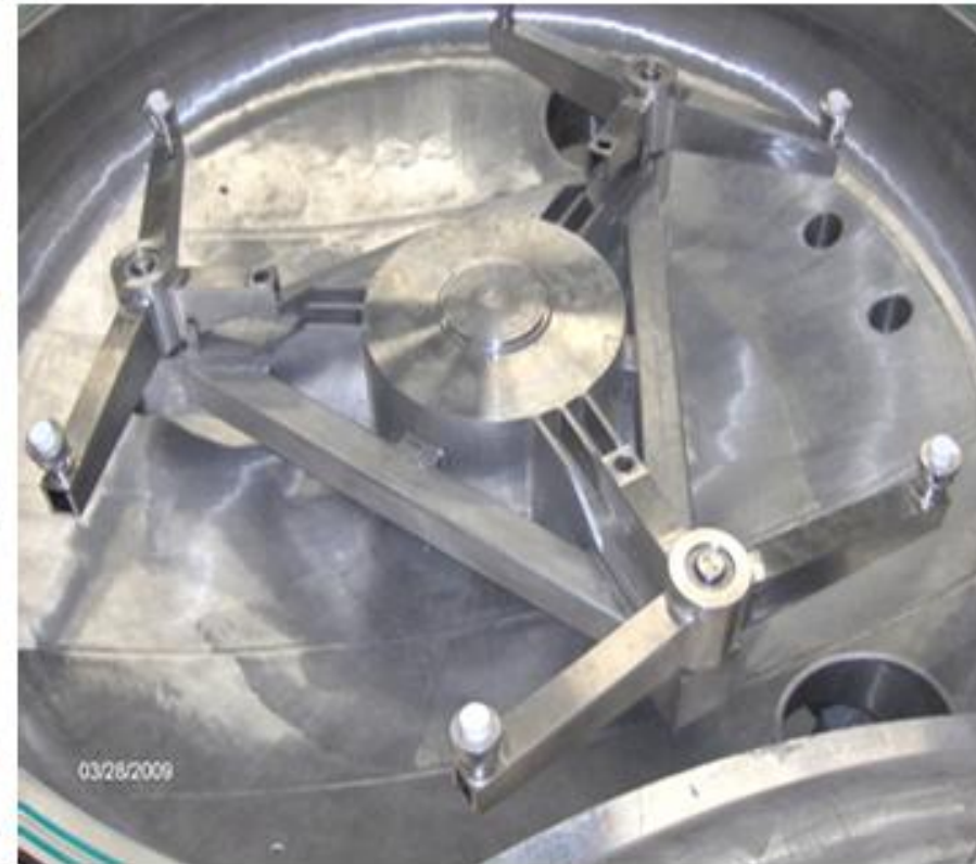
Wiffle tree with test Coupons
