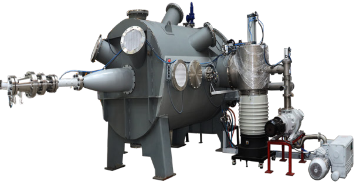
Fig.1. Mid-size Hypersonic Ludwig Tunnel, designed and manufactured by HHVTT.
