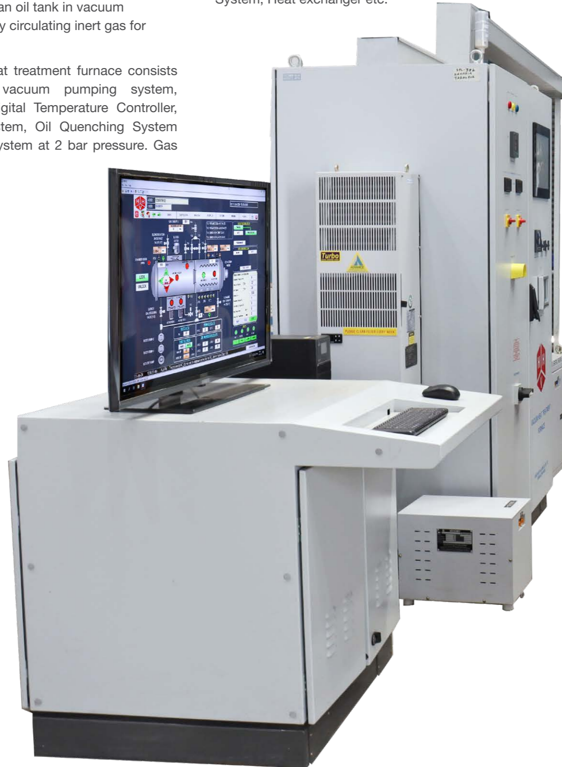
Figure 1: Vacuum Heat Treatment Furnace with Oil and Gas Quenching Facility
