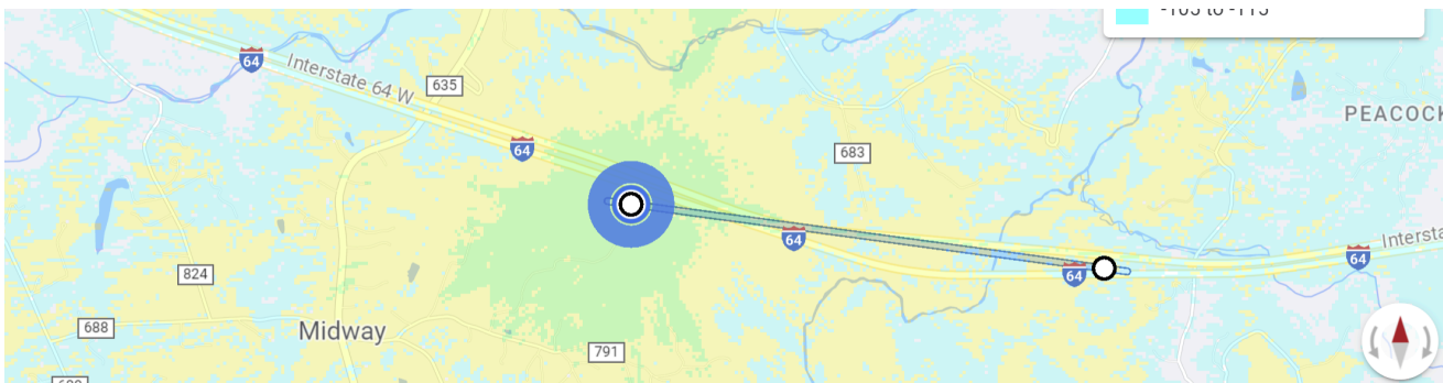
Figure 17: Example 140' Taller Tower Coverage Range with Radios on Tower
