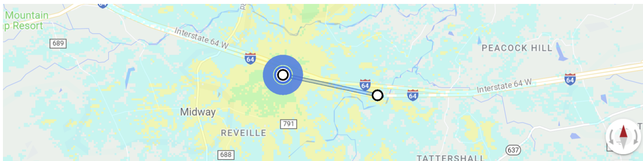
Figure 16: Example 100' Tower Coverage Range with Radios on Ground
