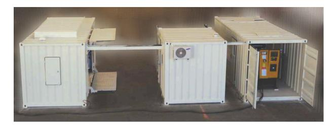
The complex is designed for flash-butt welding in stationary conditions with continuous or pulsed flashing of rails with a cross-section of 5000 up to 1000 mm<sup>2</sup> into rail weaves up to 1000 meters long during the construction of continuous (including high-speed) railway tracks with burr removal immediately after welding.
