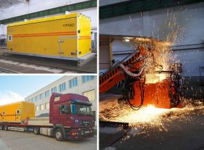
To operate the crane-manipulator, the container is equipped with rear and side opening boards, doors and hatches necessary for operation of the complex and installation of equipment. The crane-manipulator ensures that the welding machine is removed from the container and positioned at the joint of the rails to be welded. After finishing welding with a crane-manipulator, the welding machine will be returned into the container.
