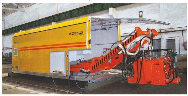
The complex is designed for flash-butt welding in field conditions with pulsed flashing of rails with cross-section of 6500-10000 mm<sup>2</sup> with burr removal immediately after welding. The complex is produced in the form of a 20ft sea container, designed for mounting both on the truck base and on a railway platform moving by rail to the welding work
