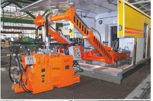
The container contains a welding machine K 922-1, a crane-manipulator, a diesel generator unit, a fire extinguishing system, a pump station, control cabinets for the welding machine and the complex, and a water cooling post.
