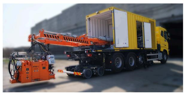
Mobile Rail-welding complex KCM007 based on rail-welding machine K922-1
