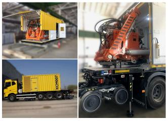
The base of the complex is a VOLVO truck chassis equipped with a railroad hydrostatic bogie drive for traveling on a rail track of 1520, 1435 or 1000 mm width.
