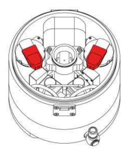
We recommend charging the batteries to full capacity one week or less before diving. Before a brief dive (up to one hour), it is permissible to store fully charged batteries for up to one month.
