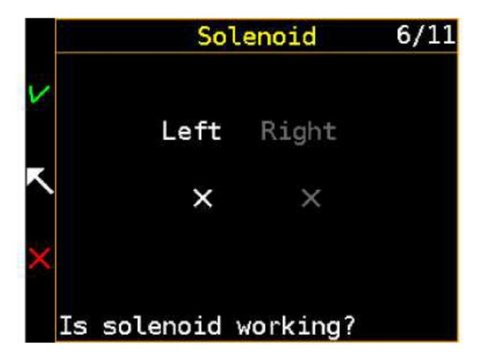
The left solenoid is repeatedly opened three times and closed in a two-seconds interval, with a 1:1 duty cycle. The expected activity of the solenoid is shown on the HS display. The right solenoid is subsequently tested in the same manner.
