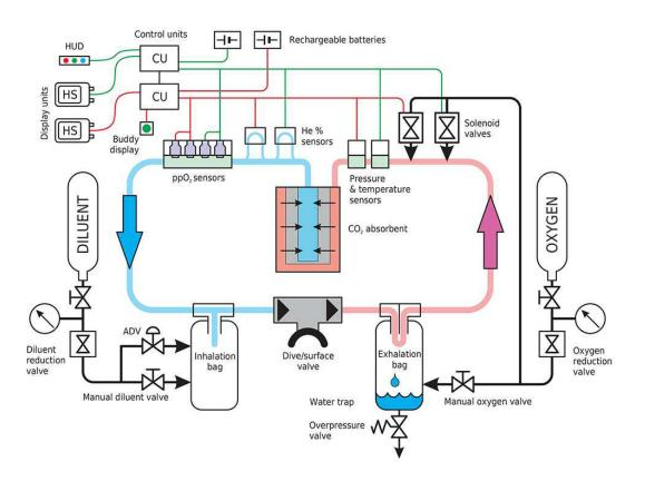
The principle of a rebreather involves in recycling the breathing mixture. Carbon dioxide is removed from the exhaled mixture and is again prepared for the next
