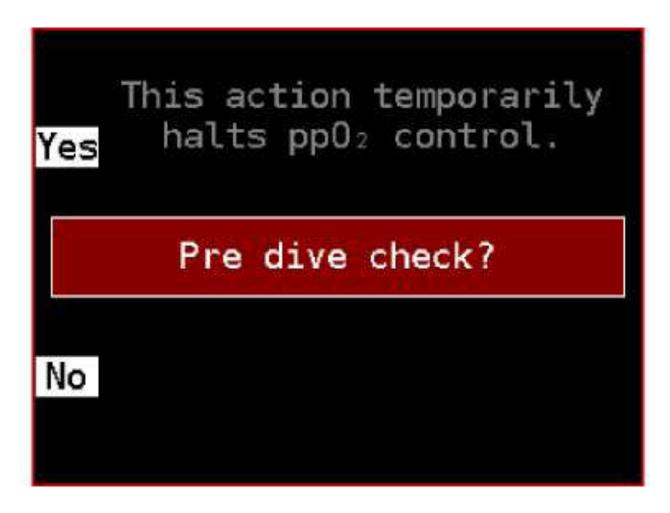
The pre-dive inspection (PDI) procedure can be started in surface mode. Testing is conducted immediately before the dive with a fully assembled rebreather with the control units switched on.
