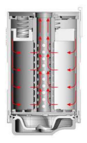
The CCR Liberty uses a radial scrubber. The breathing mixture flows from the outside to the center of the scrubber cartridge.
