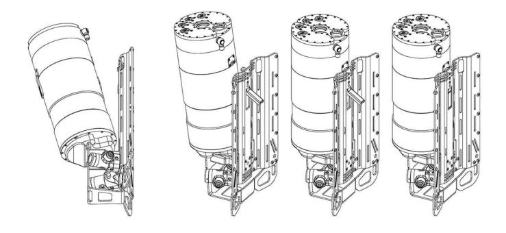
The CCR Liberty's integrated stand, which serves as a lumbar support, is intended for setting the rebreather on a hard, level surface with sufficient rigidity. Always secure the standing rebreather to prevent falling.
