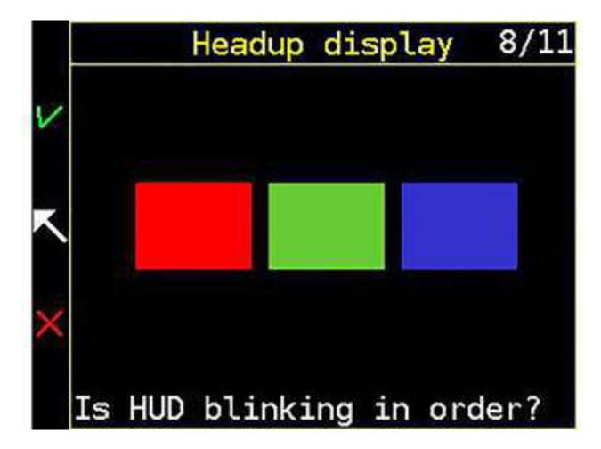
The diodes light up in blue, red, and green in three steps. At the same time, the HS displays which colors should light up on the HUD. Three different color combinations are displayed three times so that each of the three colors of the RGB spectrum are tested.
