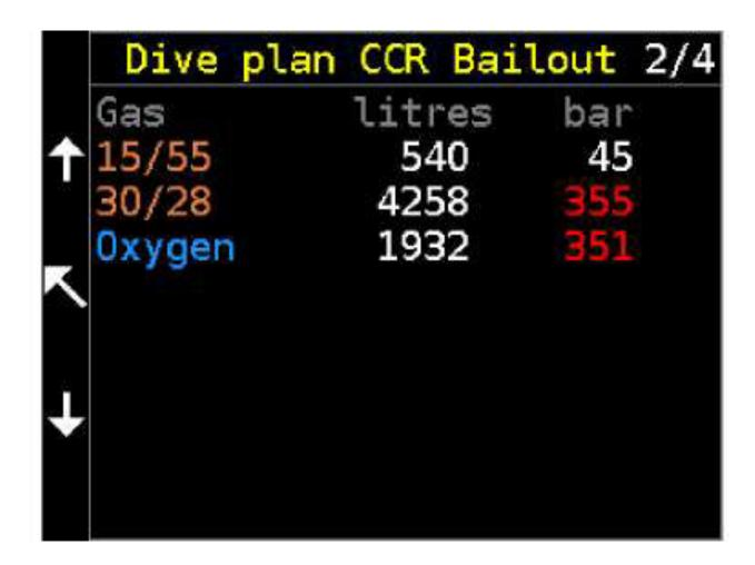
The second Bailout screen – "gas management" shows the individual gases used and their consumption in liters (cu ft) and bars (PSI). If the pressure exceeds the limits of the cylinder, it is red. In this case, it is necessary to add another gas to the dive plan. If you do not have additional gas available, shorten the bottom time or reduce the target depth.
