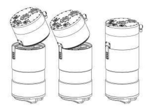
When mounting the head, push the scrubber canister pin into the opening on the head, and close the head.
