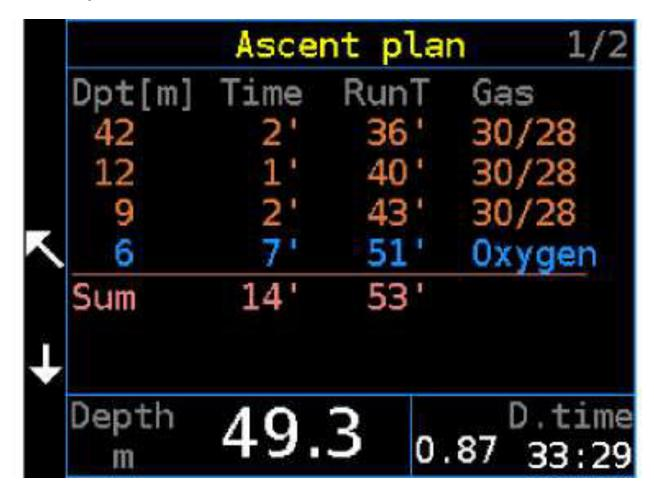
In any diving mode, you can view the current ascent plan with the entire decompression course. Although Decompression is shown on the Liberty using the depth of the decompression ceiling and time to surface, the Ascent plan is displayed
