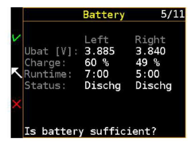
Both batteries are stressed with an artificial load caused by an intentionally increased power consumption by the processors, connected solenoids (without using energy-efficient control), vibration motors, and the maximum brightness of the HS display. After completing the test, the status of both batteries (%) (including the estimated duration of the batteries in dive mode) are shown.
