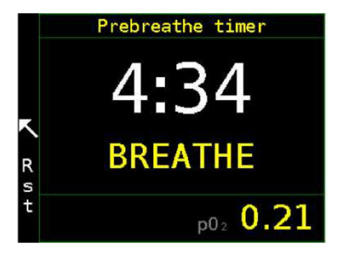
While the first function can be easily verified by observing oxygen sensors during breathing from the unit, testing the absorber functionality should only be performed under the conditions listed below, while also listening to your body's reactions. Even after a 5-minute pre-breathing from the unit, it is not guaranteed that a poorly filled or missing absorber has been detected.
