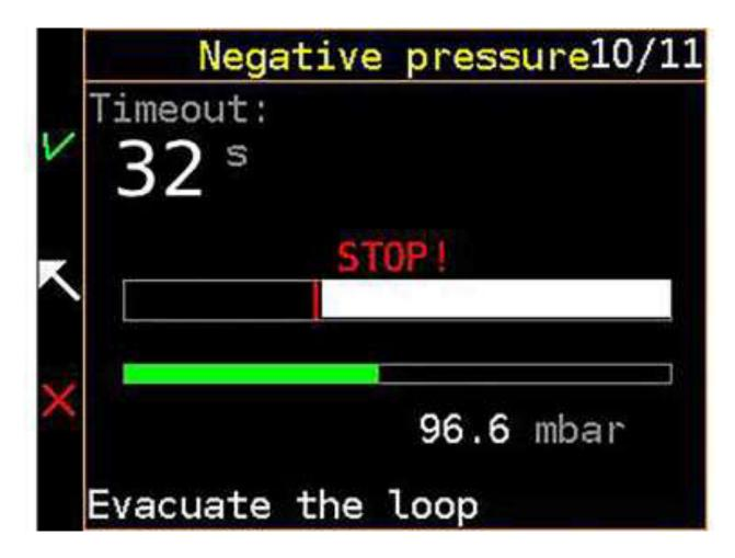
The purpose of this test is to detect possible leakage in the breathing loop, which appears when the pressure in the loop is lower the ambient pressure. The test is conducted immediately before diving, with a fully assembled rebreather.
