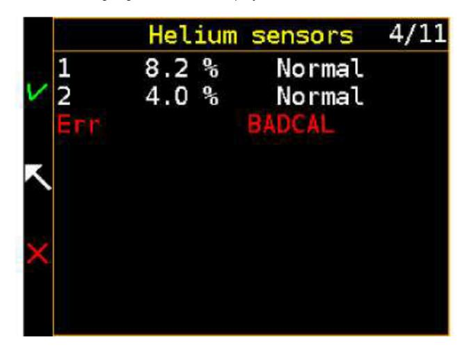
The purpose of the Helium-sensor test is to detect if the sensors are calibrated or if they show normal values. The picture shows a bad or missing calibration detected during the test. The test is automatic. Confirmation by the user is required only in the event that the test result is negative.
