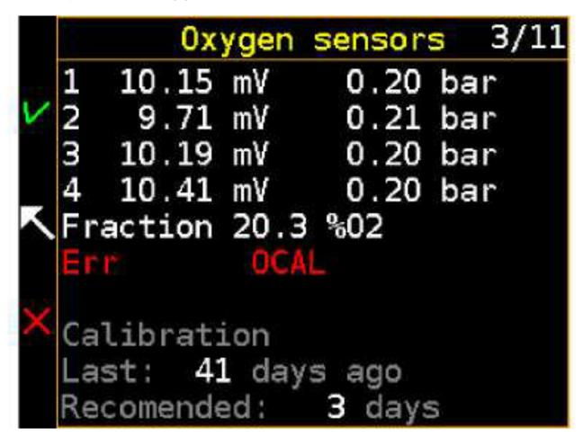
The current values of the individual sensors are shown on the display in millivolts  $(ppO_2 \text{ values are displayed in bars})$  using to the most recent calibration.
