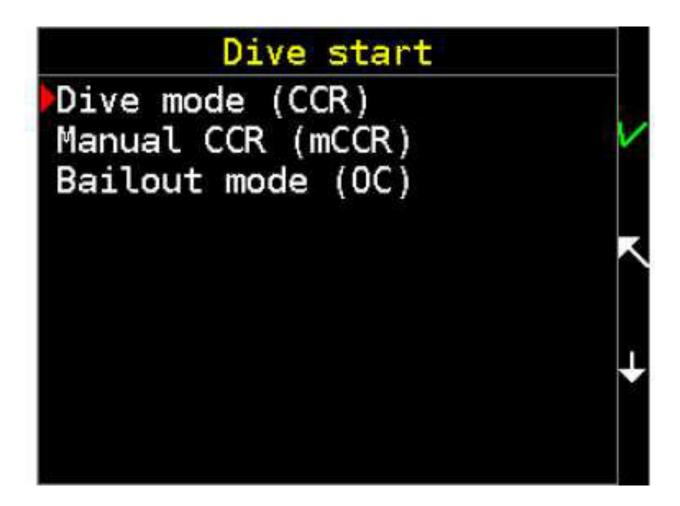
In the menu the user can switch from surface mode to the CCR, manual CCR, bailout and standby modes.
