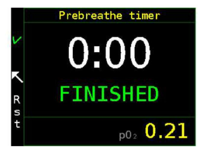
In the lower right corner, the average  $ppO_2$  is displayed. All sensors and other values can be monitored on the second handset, where all dive mode screens are accessible. If pre-breathing is interrupted, the countdown can be reset with the lower key.
