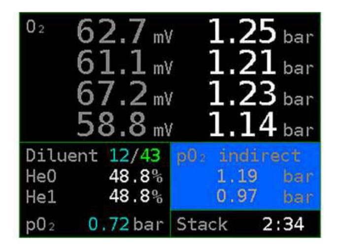
To switch between the different screens in surface mode, press the top button. Both  $ppO_2$  and sensor voltage can be read. If a sensor is not an operational state (not connected, offline, error, excluded, disabled, uncalibrated), the appropriate tag appears instead of the  $ppO_2$  value.
