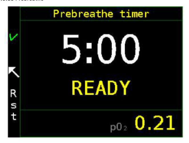
Pre-breathing the unit has a major impact on the safety of the dive. We strongly recommend performing a pre-breath before and in between every individual dive. Pre-breathing is not related to the start of the scrubber's chemical reaction, but to **verify** the important functions of the device before the dive, in particular, the ability of the device to maintain  $ppO_2$  at the setpoint and the functionality of the sorbent.
