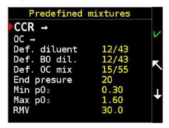
In mixture settings, note the Respiration minute volume expressed in liters per minute (l / min) or in cubic feet per minute (cu ft / min). We recommend that you choose a sufficient reserve for a crisis situation. During a  $\rm CO_2$  hit (hypercapnia), 78 a diver's ventilation can exceed 50 l / min (1.8 cuft / min). For details on the planner settings, see Menu / Setup / Decompression / Planner setup
