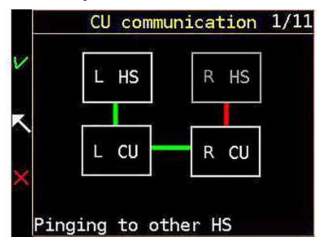
A communication test between the control units and the peripheral devices is automatically started at the beginning of the pre-dive inspection.
