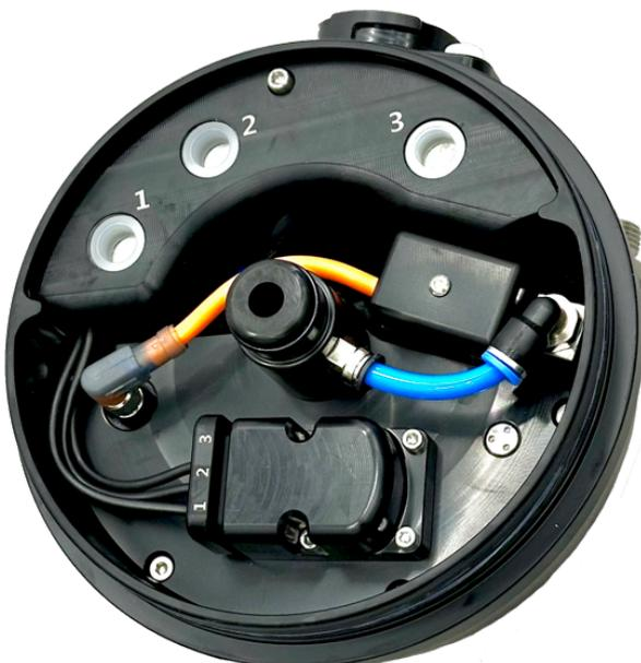
The CCR head is the heart of the FX CCR, which contains the control electronics, the solenoid valve for controlled dosing of oxygen, the removable sensor holder carrying three oxygen sensors, watertight connectors for connection of the external battery case, primary controller and Head-Up Display as well as the BN3 connector with unique Click-Lock bayonet for quick and easy connecting of the inhale counterlung.
