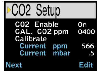
In CAL. CO2 ppm set the actual CO2 ppm of the currently used calibrating gas according to which ppm was set.
