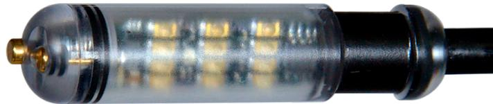
The main feature of the Head-Up Display (the HUD) is to show the current status of ppO<sub>2</sub> in the breathing loop as well as ppO<sub>2</sub> alarms to the diver.
