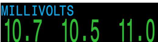
Shows the raw millivolt outputs of external PPO<sub>2</sub> cells. This is important information used to understand the O<sub>2</sub> cell output behavior over time.
