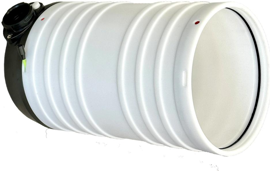
The Scrubber Canister is made from durable Delrin tubing and has grooves for O-rings and locking strings. The Canister has the fitted Canister Lid which is equipped with the water trap disk, sealed with an o-ring. The water trap disk is a pull-out if it's needed for cleaning. The Lid is secured in the Canister by the string which is inserted through the hole in the Canister into the corresponding groove.
