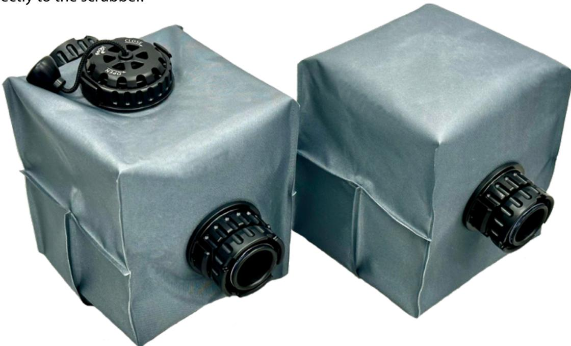
The Counterlungs are connected to the Canister and FX Head via the click-Lock Bayonet Couplers with different keying on each bayonet connector, making it impossible to connect the counterlungs incorrectly.
