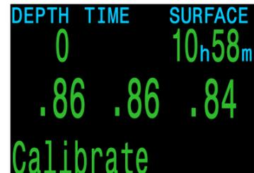
If you need to change the calibration gas FO2, do this in the System Setup → O2 Setup menu.
