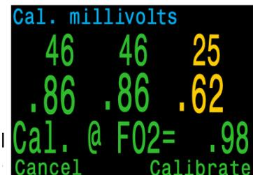
Good sensors should be in the range of 35 - 65 mV at sea level in 100% oxygen. A sensor will fail calibration if not in the range of 30mV to 70 mV. This allowable range scales automatically with changes to FO2 and barometric pressure. If outside the allowable range, a millivolt reading is shown in **yellow**.
