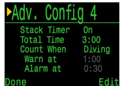
The current stack timer count used and remaining will be available as an info screen when the stack timer is enabled. The stack timer can also be reset from the main level menu. The stack timer cannot be reset during a dive.
