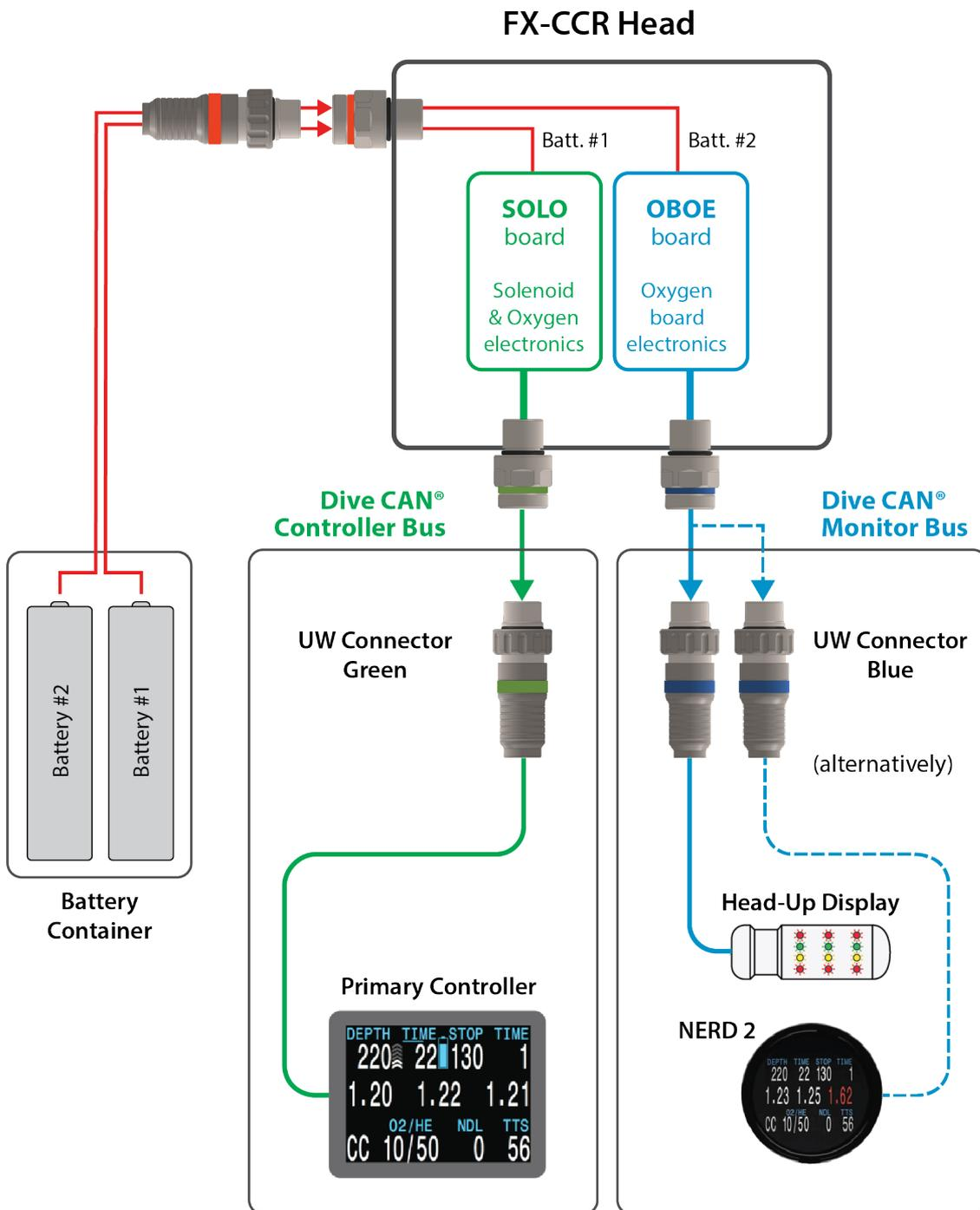
DiveCAN® connections allow rebreather components to communicate.
