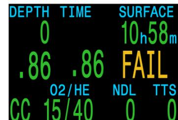
Once the calibration completes, a report will be shown. This shows which sensors passed calibration, and the value of the expected PPO2 based on barometric pressure and the FO2.
