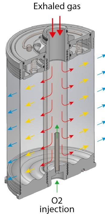
The FX CCR is equipped with the radial scrubber placed in the Scrubber Canister. The breathing gas passes through the center tube to the outer tube of the scrubber, then it flows along the outer tube to the FX head. The FX scrubber has capacity of 2,2 kg / 4,9 lb of soda lime with typical operating time of up to 4 hours.
