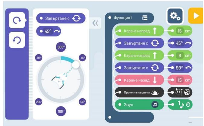
Fig. 6 Determining rotation angle in Photon Blocks (Expert Level)
