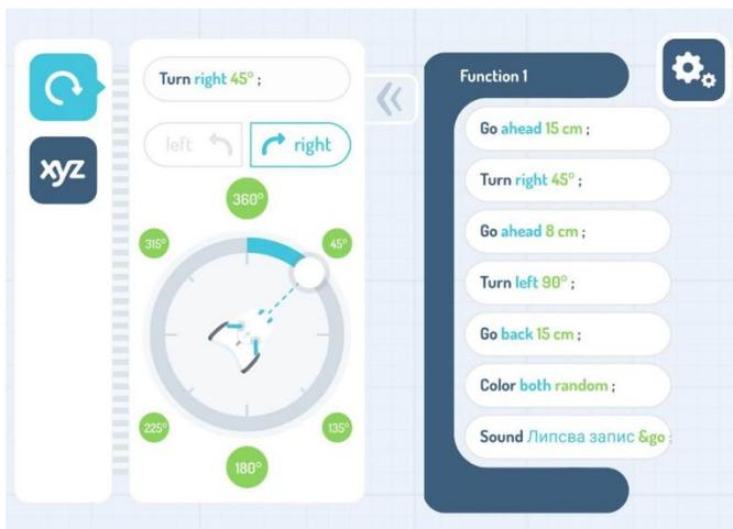
Fig. 9 Determining Direction and Rotation Angle in Photon Code (Master Level)
