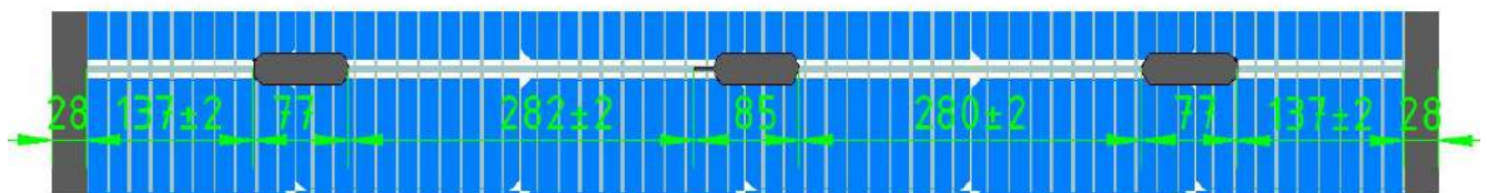
Figure 8. Position of the junction box in Blackstar B.108 and SOLID Framed B.120 Series modules
