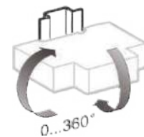
Indifferent position of installation.
